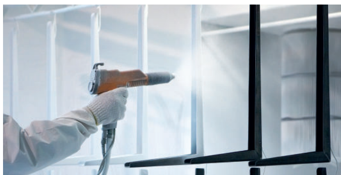
Powder coating: Application of powder paint in the spray booth.
