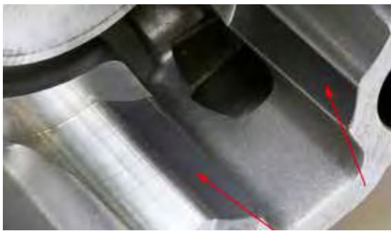
Aluminium component with partially coated surfaces
