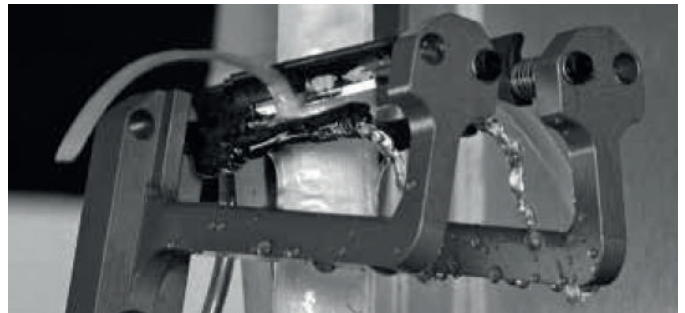
HART-COAT®-GLATT coated (25 µm) lever and knife carrier for asparagus peeling machines. The layer protects against corrosion and provides improved cleaning and wear properties.
