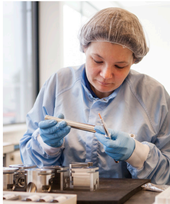
A solder assembly in which a heating wire is vacuum soldered to a product.
