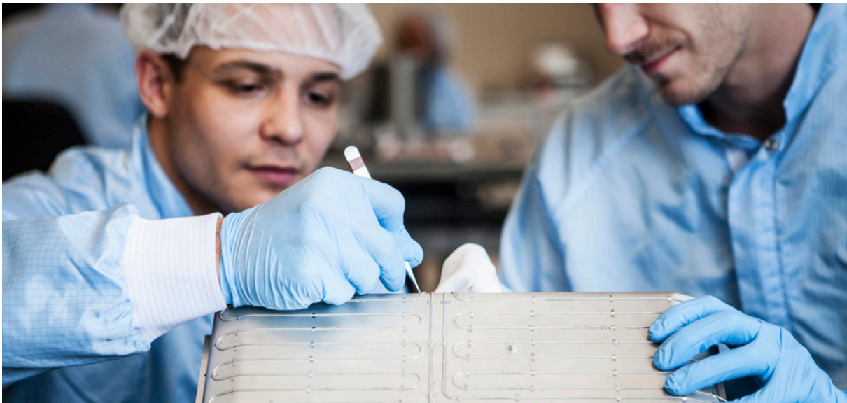
A solder assembly in which a heating wire is vacuum soldered to a product.
