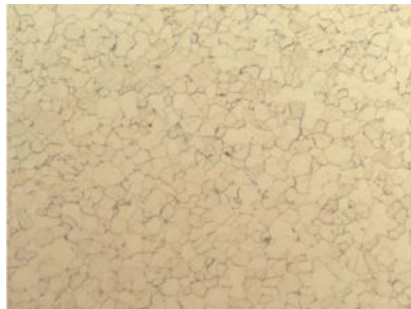
Microstructure after annealing
