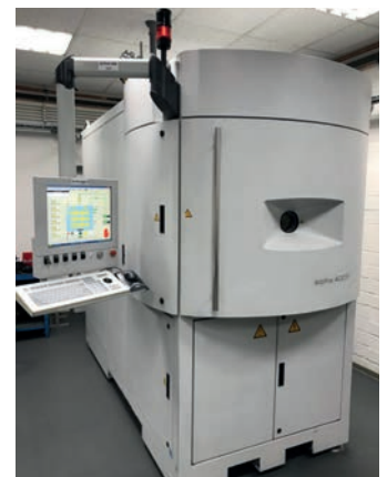
PVD system with duplex unit (working volume D 400 x 500 mm).
